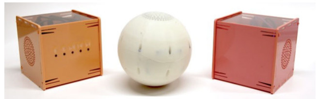
Figure 2: Three designs of speakers. Left: cube with button controls; centre: sphere; right: cube with gesture controls.
