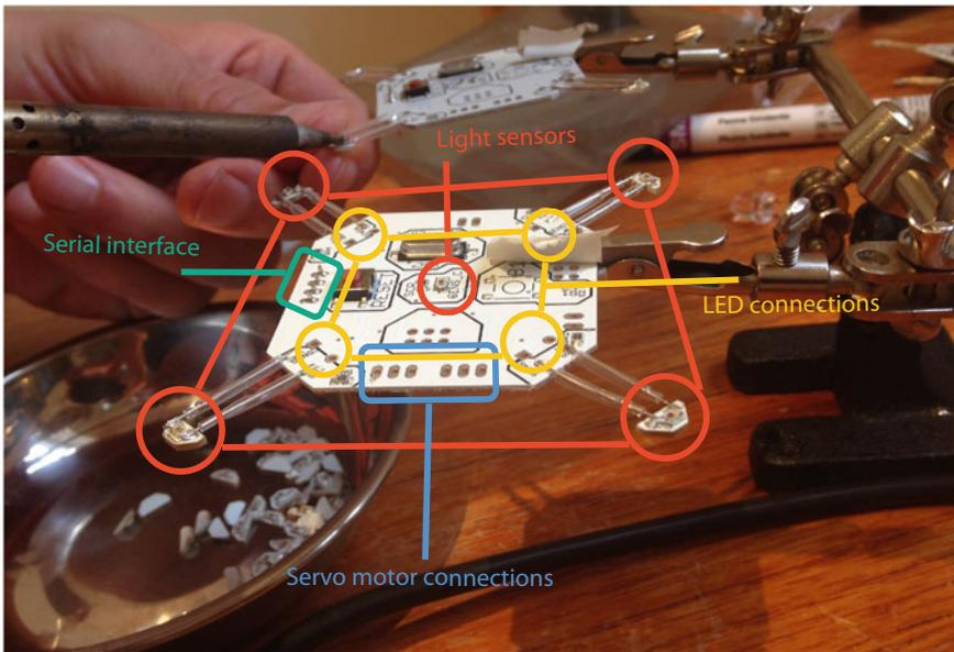
**Fig. 8.2** Printed Circuit Boards (PCBs) being assembled; image features two PCBs, a hand, soldering iron and components. The graphics feature the layout and position of components
