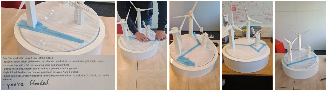
Figure 3: Incorporating a new element into the physical prototype through physical and descriptive modification of prototype
