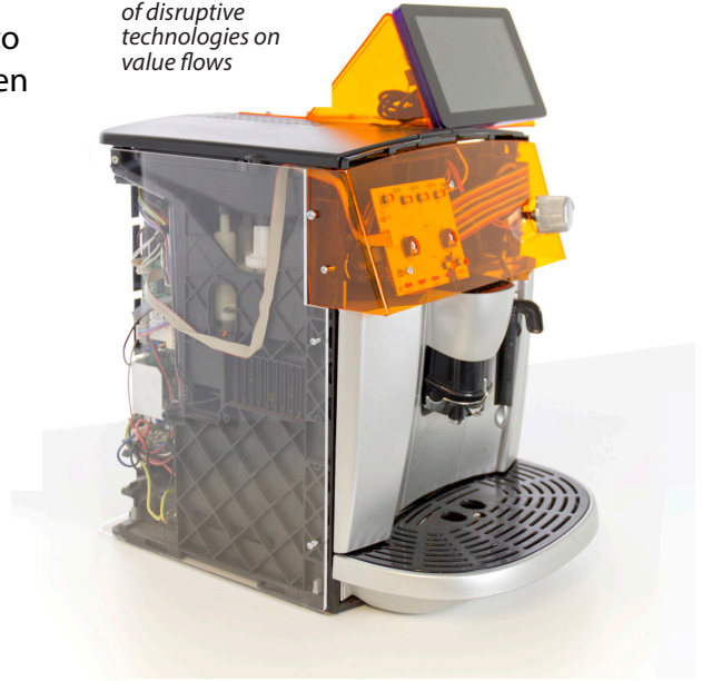
The Bitbarista, a hacked Delonghi home coffee machine. Image credit: Mark Kobine
